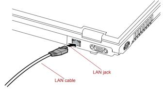
Figure 4-10 Connecting the LAN cable
